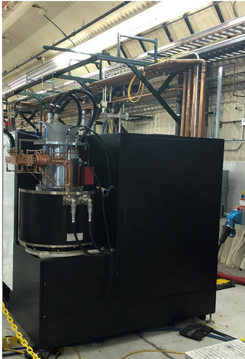
Figure 1: Photographs of the CERF-NM: the control station and the lead box for radiation protection (top); the 5.712 GHz Canon klystron (bottom).
