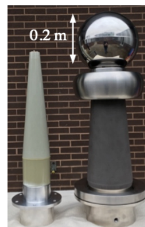
Figure 4: Picture of the tapered epoxy receptacle (left) next to the 500 kV doped alumina insulator with triple point junction shield and spherical electrode (0.2 m diameter).
