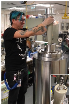
Figure 5: Postdoctoral fellow Gabriel Palacios-Serrano installing the modified epoxy receptacle to the SF 6 reservoir assembly on top of the testing chamber. Inset: Close-up view of the spring attached to the end of the epoxy receptacle.
