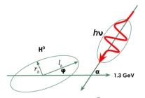
Figure 2: Crab-crossing scheme of H<sup>0</sup> beam photoionization by laser pulse.
