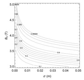
Figure 1: Stripping efficiency of 2p excited state in a 1.3 GeV hydrogen beam in a magnetic field (1).
