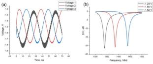
Figure 9: AC voltage bias at phase differences of 120° per ventil (left). Dependence of the Fano resonance on the applied DC voltage bias amplitude (right).
