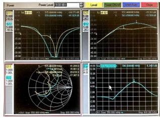
Figure 5: Measured reflection (S11, S22) (left) and transmission (S21, S12) parameters, showing isolation (=of 6.3 dB (right) in the 2-port isolator prototype.
