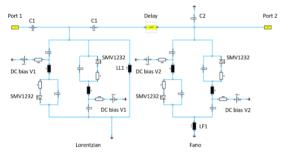
Figure 2: The RF design of this nonreciprocal Fano-Lorentzian-based isolator.
