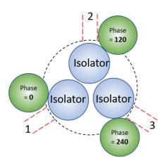
Figure 1: Modulation scheme with 120-degree phase difference between modulation sources.
