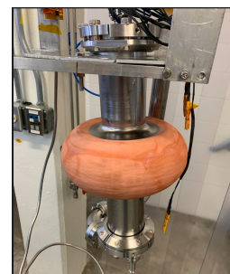
Figure 6: 1.3 GHz cavity with 8 mm thick Cu layer.
