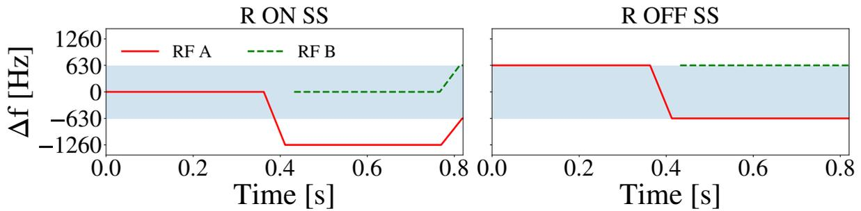
Figure 4: A comparison of the two slip-stacking schemes. Radial On-center (R ON) and Radial Off-Center (R OFF). The frequency of the two rf systems is shown.
