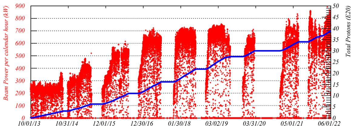
Figure 2: The hourly beam power to NuMI and the total protons delivered since the end of the long shutdown in 2013.
