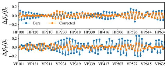
Figure 5: The difference between measured and design  $\beta$  functions before and after corrections.
