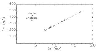
Figure 5: Electron detector signal below and above instability threshold with full, 160-bunch fill at BEPC.
