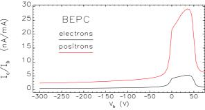
Figure 4: Comparison of detector signals for positron and electron beams (APS: 10 bunches, 20 mA, 2.84-ns spacing; BEPC: 160 bunches, 10 mA, 5-ns spacing). BEPC single-bunch results are almost identical to the multibunch case shown.
