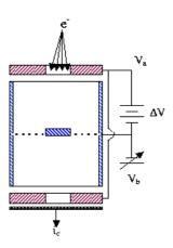
Figure 6: Schematic diagram of the Bessel Box Analyzer. The difference potential  $\Delta V = (V_a - V_b)$  determines the pass energy of the detector.
