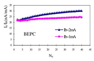
Figure 3: Electron detector current (normalized to total beam current) vs. increasing bunch number ( $N_b$ ) as a function of bunch current (bunch spacing for APS is 20 ns, and for BEPC is 10 ns). Note that the APS data is plotted on a log scale.
