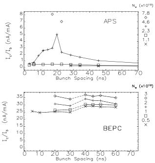
Figure 2: Electron detector current (I<sub>c</sub>) vs. bunch spacing as a function of positrons/bunch (N<sub>e</sub>), normalized to total beam current (I<sub>b</sub>) (APS: 10 bunches; BEPC: 5 bunches).
