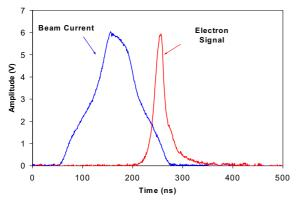
Figure 4. Electron signal compared to a 6.8  $\mu$ C beam pulse in a single pass experiment (Vrep = +25 V).
