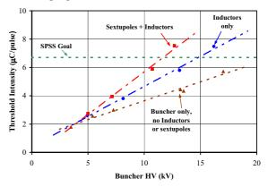
Figure 6. Effect of inductive inserts and sextupoles on the instability threshold-intensity curves.
