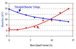
Figure 7. Instability threshold voltage and relative beam losses as a function of skew quad current for fixed beam intensity (stored charge of 5  $\mu$ C/pulse).
