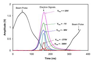
Figure 2. Electron signals during a single revolution plotted in time relation to the beam pulse.
