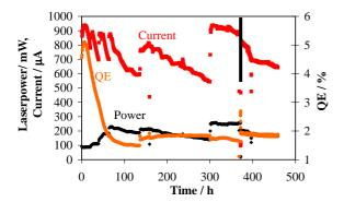
Figure 3: Behaviour of a CsTe cathode under high average current; total produced charge 1.22 kC .
