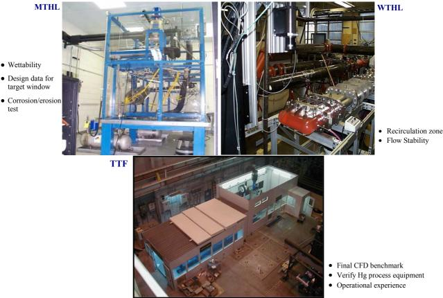
Figure 2: Experimental Facilities which are used at ORNL to carry out CFD and remote handling tests (TTF only): WTHL, MTHL, and TTF.
