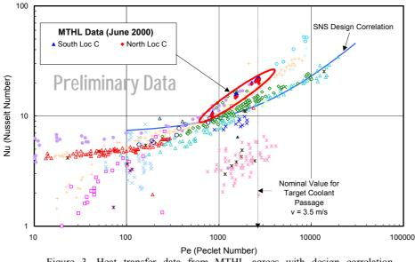
Figure 3. Heat transfer data from MTHL agrees with design correlation predicted from CFD calculations.
