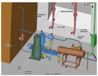
Figure 5: Hot cell arrangement for the mercury target equipment.
