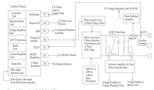
Figure 1: Monopolar I.R. P.S. Block Diagram
