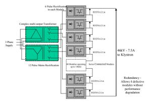
Fig 5. Thomcast Pulse Step modulator 46kV 7.5A
