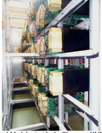
Fig 4 Modules inside the Thomcast HVPC
