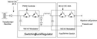
Figure 7. DTI Buck regulator and series[3]
