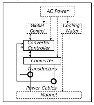
Figure 1: Power System Block Diagram
