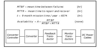
Figure 2: Definitions And Reliability Block Diagram
