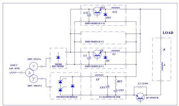
Figure 3: Basic configuration of the booster dipole power supply.
