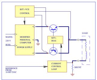
Figure 1: Block diagram of the corrector power supply.
