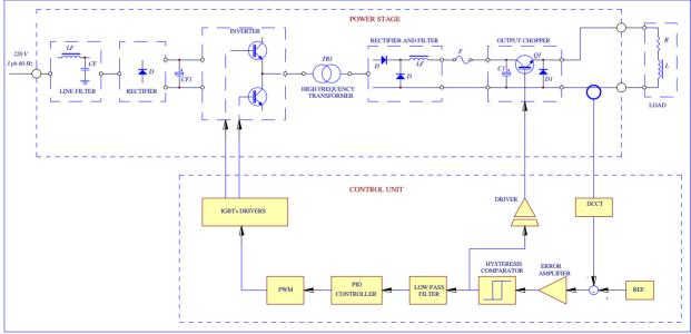
Figure 2: Block diagram of the quadrupole and sextupole power supplies.
