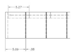
Figure 2: Ferrite blocks of injection kicker (dimensions in cm)
