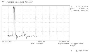
Figure 6: All-ferrite magnet with 25  $\Omega$  load @ 38 kV
