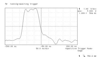
Figure 4: Current in the all-ferrite magnet (32 kV and  $16\Omega$ )
