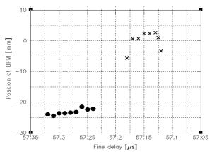
Figure 8: Beam based rise time measurement of the blue ring with one all-ferrite kicker magnet.
