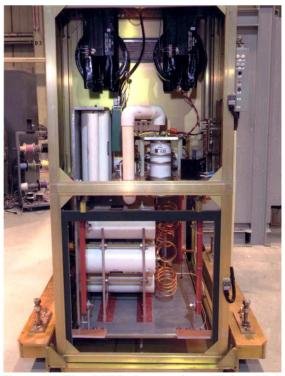
Figure 1. The RHIC Beam Abort Kicker High Voltage Modulator.
