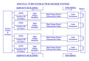
Figure 2. The SNS Extraction Fast Kicker System Layout.
