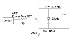
Figure 1. The Snubber circuit of the SRRC-1000.
