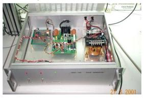
Figure 7: Internal arrangement of SRRC-1000 System.
