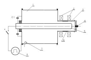
Figure 5: Scheme of the experimental setup. 1. capacitance-loaded quarter-wave resonator; 2. solenoid; 3. tungsten-wire thermionic cathode; 4. feed input; 5. central resonator electrode – diode anode; 6. working area of secondary emission cathode; 7. excitation loop/diagnostics; 8. pulsed high-voltage generator; C1 blocking condenser
