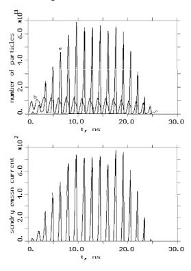
Figure 2: The dynamics of a change in the number of primary and secondary electrons in the accelerating gap and behavior of secondary emission current.
