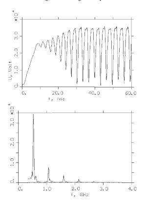
Figure 4: Behavior the voltage on magnetron gun and frequency spectrum of oscillations.
