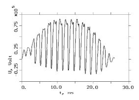
Figure 1: Behavior of voltage on magnetron gun.
