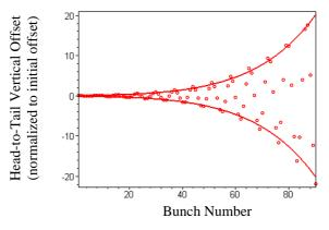
Figure 2. Estimated capacity for generating multibunch BBU in ETF. The envelope is generated analytically.
