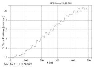
Figure 4. Vertical emittance of the bunch train (in  $\mu$ m) plotted along the ETF. The horizontal emittance is lower.
