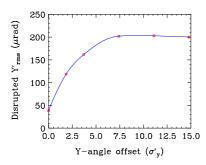
Figure 6: Disrupted rms vertical divergence at IP vs.  $\Delta y'$ .
