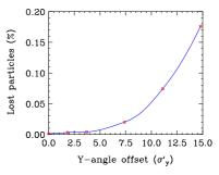
Figure 8: Particle loss in the extraction line vs.  $\Delta y'$  offset.
