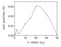
Figure 4: Particle loss in the extraction line vs.  $\Delta y$  offset.
