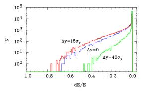
Figure 3: Energy spread at IP for  $\Delta y = 0$ ,  $15\sigma_y$  and  $40\sigma_y$ .
