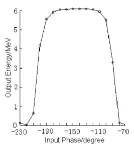
Figure 3: Energy Spectra as a Function of Input Phase.
