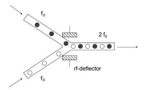
Fig. 1: Principle of funneling.
