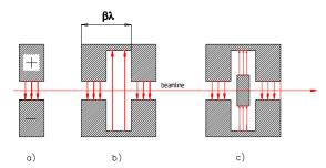
Fig. 5: Schemes of funnel deflectors. The arrows show the electric field during one period. a) a one cell one gap deflector, b) a three cell multigap deflector, c) multigap deflector with one central drift tube.
