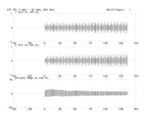
Figure 8: Beam trajectory in DTL
