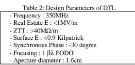
The aperture of the DTL can be optimised by iterative calculations of the shunt impedance and the beam trajectory for the optimisation. A larger aperture decreases the shunt impedance, but increases the ratio of aperture to beam size (less beam loss).
