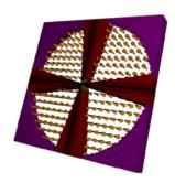
Figure 2: The 57.5 MHz 4-vane RFQ with the characteristic magnetic field of the  $TE_{21(0)}$  mode.
