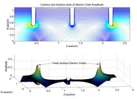
Figure 4: The contour plot and corresponding surface plot show the distribution of electric field amplitudes in a pure iris-loaded traveling-wave structure shown in Figure 2. We observe that the strongest electric field occurs at the edge of the iris. In this case,  $E/E_a$  is about 2.4.
