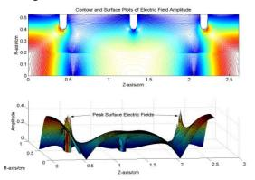
Figure 5: Contour and surface plots showing the distribution of electric field amplitude in a hybrid dielectric-iris-loaded traveling-wave structure shown in Figure 3. We can see the strongest electric field on the iris surface is about the same as the axial electric field in this case: Es/Ea is about 1.01.
