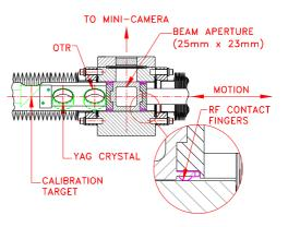
Figure 6: Built-in beam aperture in flag actuator.
