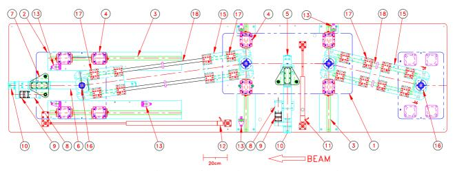
Figure 2: Motion stages of the APS bunch compressor – plan view.
