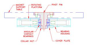
Figure 3: Bunch compressor pivot assembly.
