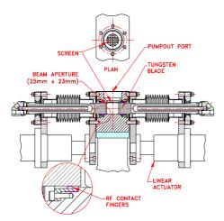
Figure 5: RF contact fingers for the scraper aperture.
