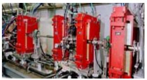
Figure 4: Bunch compressor in APS linac.
