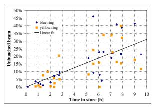
Figure 2: Unbunched beam as a function of store time.
