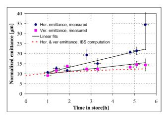
Figure 5: Transverse emittance measurements as a function of store time. Note that measurements were taken during different stores.
