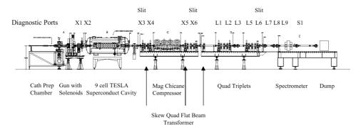
Figure 2: Layout of the FNPL photoinjector as related to this experiment.
