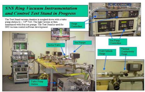
Figure 1. The SNS Vacuum Control Test Chamber.
