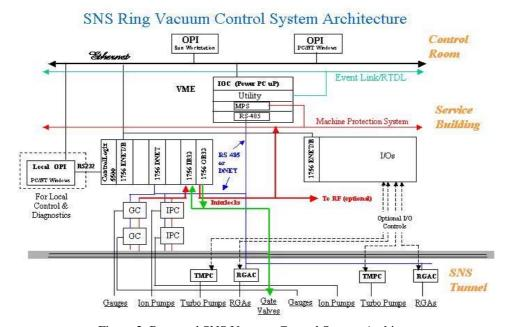
Figure 2. Proposed SNS Vacuum Control System Architecture.
