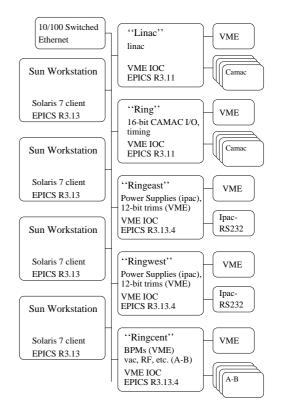
Figure 1: Proposed hardware layout for the Duke Storage Ring control system.
