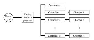
Figure 2. Block diagram for simplified timing-system dependencies. In contrast with Figure 2 the accelerator/storage ring and the chopper controllers all operate as slaves. No chopper enjoys a special status as the master chopper.
