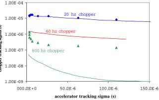
Figure 3. Predictions (lines) and measurements for chopper performance as a function of the coupling to the power grid.
