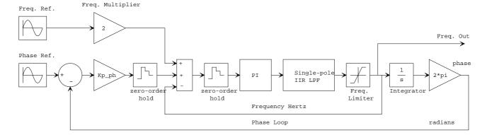
Figure 3. MATLAB/Simulink model used to design and program the DSP.
