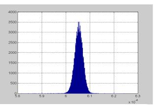
Figure 5. Level 7. Histogram of the time interval between the zero-crossing and reference output signals.
