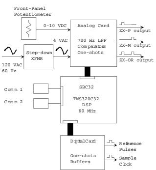
Figure 2. Block diagram of the timing-reference generator hardware.
