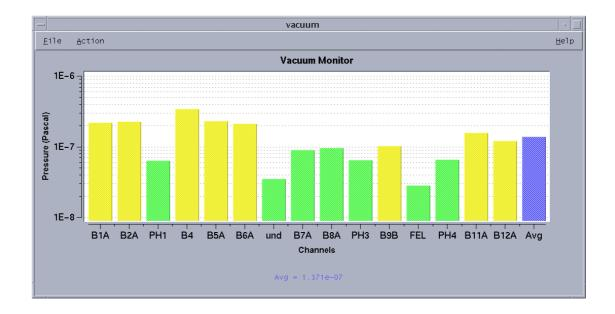
Fig. 2 the screen of HLS storage ring vacuum monitoring system
