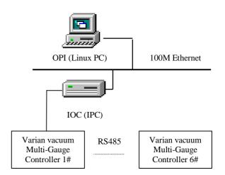
Fig.1 Structure of storage ring vacuum monitoring system.
