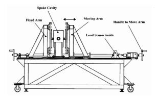
Figure 1: Room Temperature Test Set-Up.
