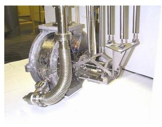
Figure 2: ANL cavity set on the vertical cryostat insert.
