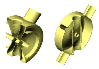
Figure 2: This is a cut-away view of the final cavity geometry with optimized spoke shape, all attached ports, and the selected end-wall geometry.
