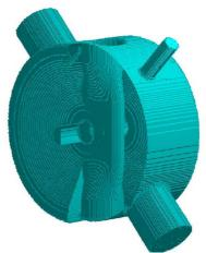
Figure 1: This figure shows a cut-away view of the MAFIA [4] model of the optimized spoke resonator. This model also includes coupler, cleaning and RF pickup ports, which are discussed later.
