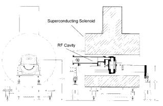
Figure 5: Layout of the high power test of the 805 MHz pill box cavity at the Lab G in Fermilab.
