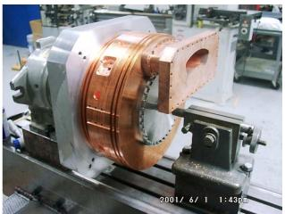
Figure 4: The single cell pillbox cavity is being fabricated at the Univ. of Mississippi. This photo shows the copper cavity body attached with the kidney shaped coupler.
