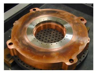
Figure 3: A stainless ring is brazed into the copper body of each half of the cavity. This photo shows the s.s. ring before it was put into hydrogen oven at Alpha-Braze a company in Fremont, California.
