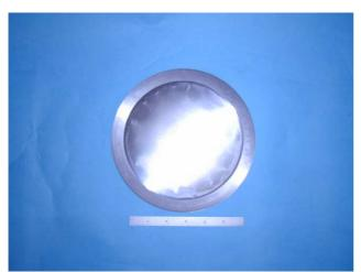
Figure 2: The Be window: a 127  $\mu$ m thickness Be foil (IF-1) is sandwiched between two annular Be frames (PS-200) the fill line to the fill between the annular be frames (PS-
