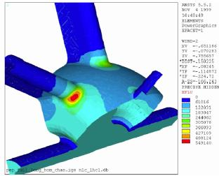
Figure 5. Surface power loss on proposed NLC cavity.
