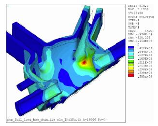
Figure 6. Von Mises stress in the cavity body.
