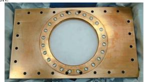
Figure 10. Finished window in waveguide flange.
