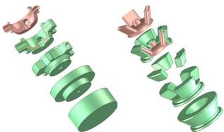
Figure 8. Development of body and lid from forgings.
