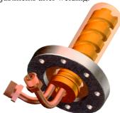
Figure 12. Plunger type tuner with spiral cooling channel.
