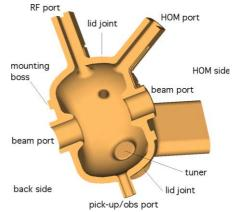
Figure 7. Section through two main pieces of cavity.
