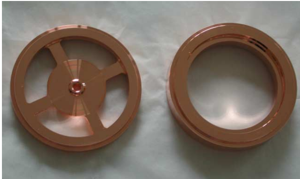
Figure 6: OFC model of the washer and disk
