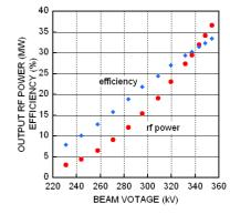
Figure 9: Saturated rf output power characteristics.
