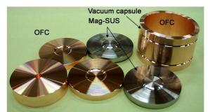
Figure 5: Machined parts pf PPM stack before assembly. They are stacked together and loaded into the vacuum capsule.
