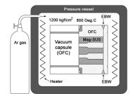
Figure 6: HIP diffusion bonding process.
