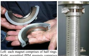
Right: assembled PPM magnets comprises of 24 modules.
