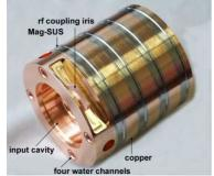
Figure 7: The diffusion bonded PPM stack. The input rf-cavity, a coupling iris, the beam hole and four water cooling channels were machined after the HIP bonding.
