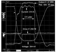
Figure 8: Output rf power, beam voltage and drive rf power waveforms.
