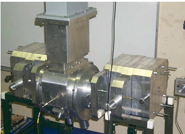
Figure 4. CCL aluminum model of bridge coupler between two 4-cavity segments and connected to the waveguide.
