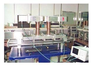
Figure 2: Experimental low-power RF setup for dimensioning the connecting waveguide
