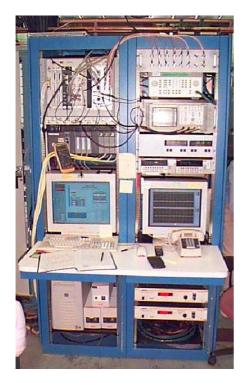
Figure 4: Instrumentation and data acquisition racks for SNS FPC RF processing
