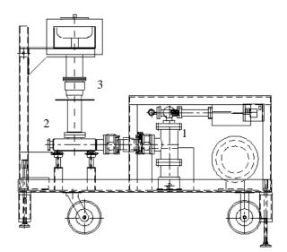
Figure 1: The FPC test cart includes a pumping unit (1), a connecting waveguide (2) and a coupler pair (3).
