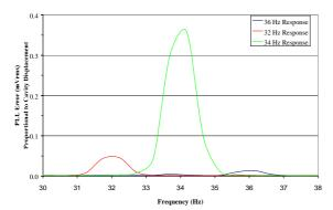
Figure 4: Swept Sine Responses, 32, 34, 36 Hz Vibration.
