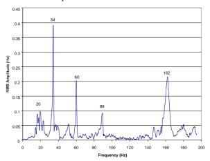
Figure 6: Cryomodule Impulse Response.
