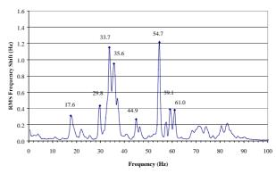
Figure 2: Cryomodule Response, Background Vibration.
