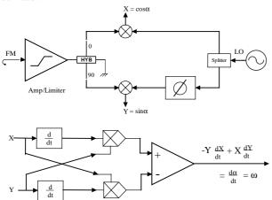
Figure 1: Cavity Resonance Monitor Block Diagram
