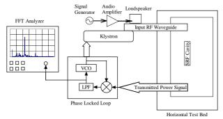
Figure 3: Swept Sine Test Setup.
