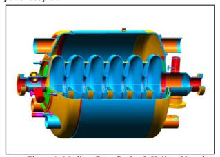
Figure 1. Medium Beta Cavity & Helium Vessel
