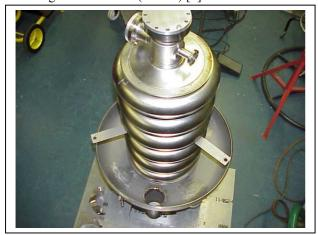
Figure 3. Cavity with Center Supports & Head
