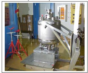
Figure 4. Cavity & Titanium Helium Vessel
