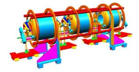
Figure 4: Cavity String Components Inside the Spaceframe Situated on Tooling
