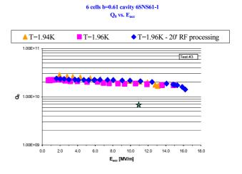
Figure 3: Medium Beta Cavity Performance
