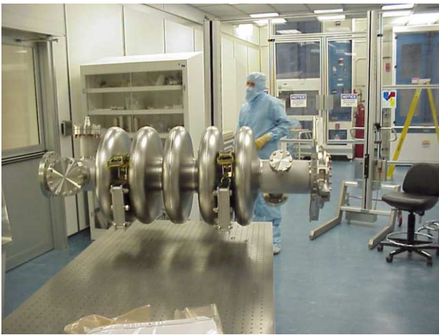
Figure 4. Preparation for RF Testing at JLAB
