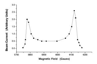
Fig. 7 Energy spectrum by magnet filed scanning
