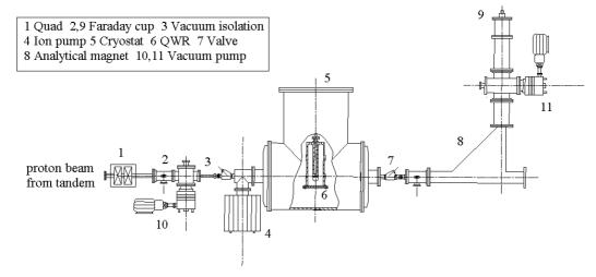
Fig. 6 Layout of proton beam accelerating structure
