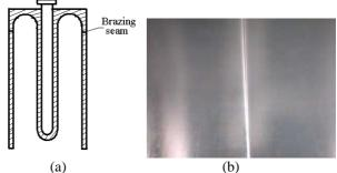
Fig. 5 Brazing seam on QWR (a) and niobium film near the seam (b)
