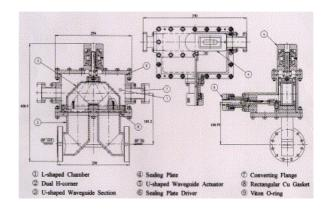
Figure 1: U-type waveguide valve
