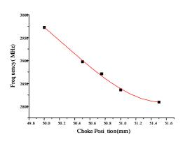
Figure 2: Relation between choke position and resonant frequency
