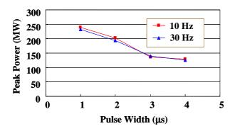
Figure 8: Maximum allowable power level of waveguide valve
