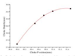
Fig.3. Relation between choke position and choke depth (d=1 mm)
