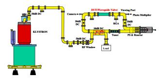
Figure 5: Layout of high power test for waveguide valve
