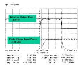
Fig. 6. Waveform of klystron output and Choke flange input
