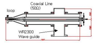
Figure 1. Drawing of the coaxial-type input coupler.
