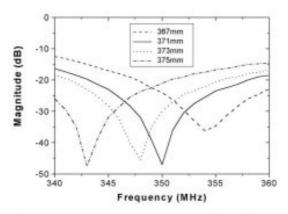
Figure 3. Return loss versus the position of short plate of the coaxial line.
