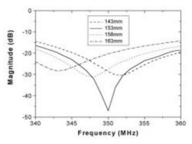
Figure 2. Return loss versus the position of short plate of the waveguide.
