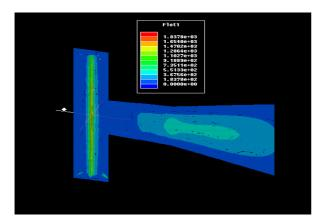
Figure 7. Electric field distribution in the RFQ and input RF coupler
