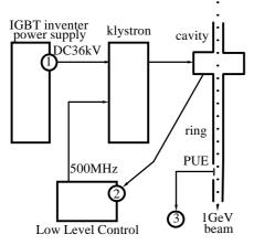
Figure 2: The ripple of DC voltage was measured at the point (1). The phase error of the 500MHz in the cavity was measured at the point (2), PLL signal of the low level control. The phase ripple of the beam is measured using the beam signal piced up from an electrode set at the beam pipe, that was the point (3).
