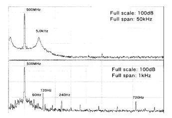
Figure 3: Side bands of the rf frequency of the beam signal, point(3) of Fig.2.
