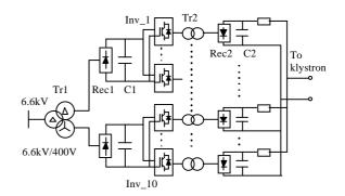
Figure 1: Configuration of a crowbarless power supply.
